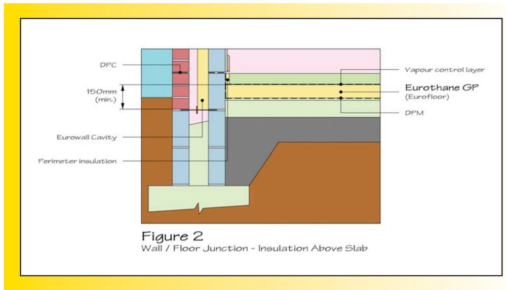
Insulating above the slab allows a rapid thermal response and is more suited to an intermittent heating regime. This method of construction is equally suited to cast in-situ concrete floors, beam and block floors and pre-cast concrete floor units.
