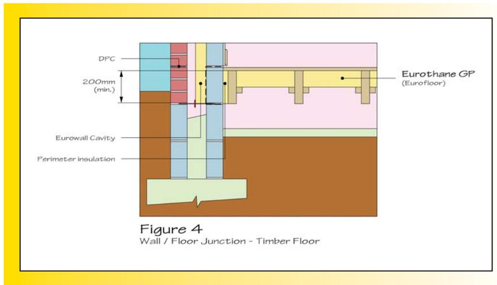
Insulating below a timber floor allows an extremely rapid thermal response and is more suited to an intermittent heating regime.
