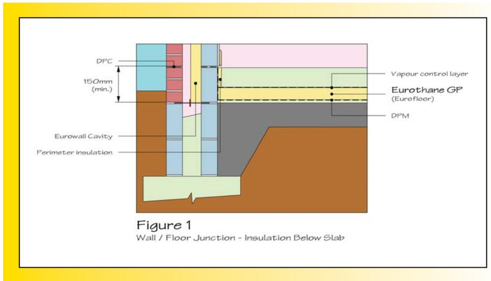
Insulating below the slab allows its full thermal mass to be utilised however its thermal response will be slow and is more suited to a continuous heating regime.
